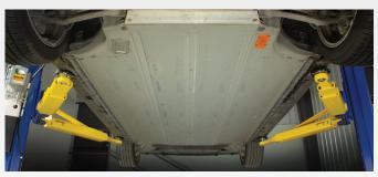
Reach small, specific pick-up points on EVs with the needed clearance to remove propulsion batteries.
